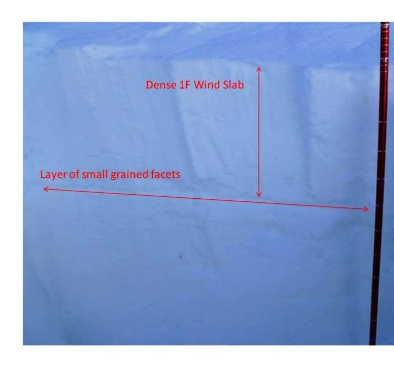
A dense wind slab sitting over a layer of small grained facets allowed the flanks of this slide to propagate outwards lower in the path. The primary weak layer for this avalanche was weak facets around a rock outcroppings near the top of the slope. The thin layer of facets in this photo required the heavy load of avalanche debris to break and is not a major concern by itself. Photo: GNFAC
