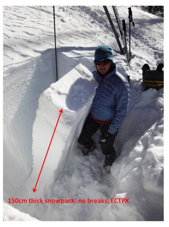
In a SW facing pit near Taylor Fork, I was able to peel this slab away after it did not break with an Extended Column Test. This slab is strong and has no weak layers that are fracturing. Model: Genevieve Chabot. Photo: GNFAC
